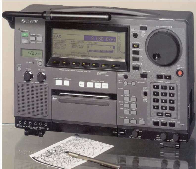
Figure 11.5: Modern receiver Sony CRF-V21 for WEFAX and RTTY reception equipped with printer.
